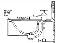
Air Gap – the area between the top of the filled container or vessel and the bottom of the faucet.
