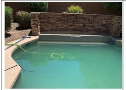
Leaving your hose end in a "pool" of water without the proper backflow preventer could cause the water in the "pool" to backflow into your home system or even into the main water supply.
